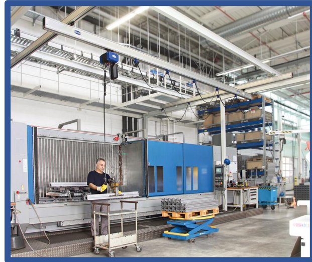
Cantilevered Track & Hoist
