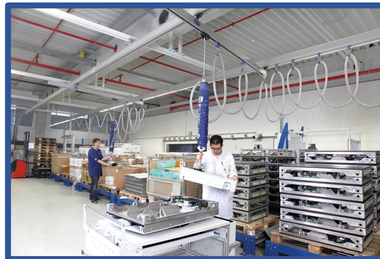
Track System & Vacuum Lifter
